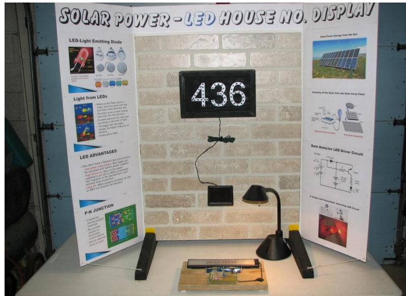
Figure 11 The completed street number display unit.
